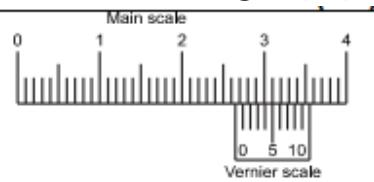
Ans: Least Count of Vernier Callipers: Least count of a Vernier Callipers is the difference between one main scale division (M.S) and one Vernier scale (V.S) division. Hence,
